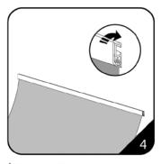
4. Slide the top of the graphic under the lip (it should allow for approx. 3/8" or 1cm insertion) and close the lip to secure the graphic.
