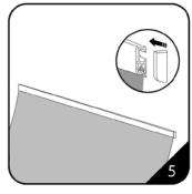
${\bf 5}$  .Then finish the top by re-attaching the plastic end caps.
